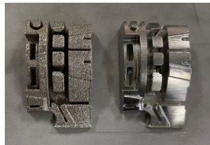
Fig. 1. Sintering and milling time comparison between conventional and upgraded machine
